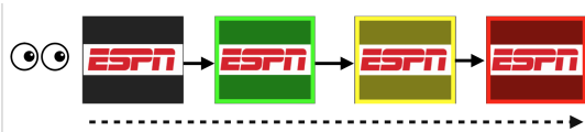
Figure 1. Gradual transition of button state, as dwell duration increases for 16 icons. The order of these tasks are randomized, but all 3 groups go through the same tasks for every session.
